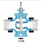
Normally Closed Valves are used for COOLING, so the valve stem opens (in-to-open) as the control signal (temperature) increases.
