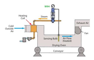
**W94** Valve used to regulate the temperature of the air flow through an air heating duct. The sensing bulb is installed toward the end of the heating duct and will sense the temperature of the air flowing past the heating coils. When air temperature is below the set point, the valve will open to allow more steam through to the coils to heat the air passing through the duct. Once the desired air temperature is achieved, the valve will begin to modulate closed to maintain the air temperature.
