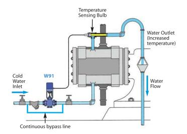
When the Sensing Bulb is mounted remotely from the actual point of Cooling (as shown), the water MUST continue to flow so that the sensing bulb can sample the product temperature of the unit being cooled. Without continuous water flow, the temperature control valve will never turn on, causing the unit to overheat. The bypass line provides a minimum continuous flow when temperature set point is achieved and the valve is closed.
